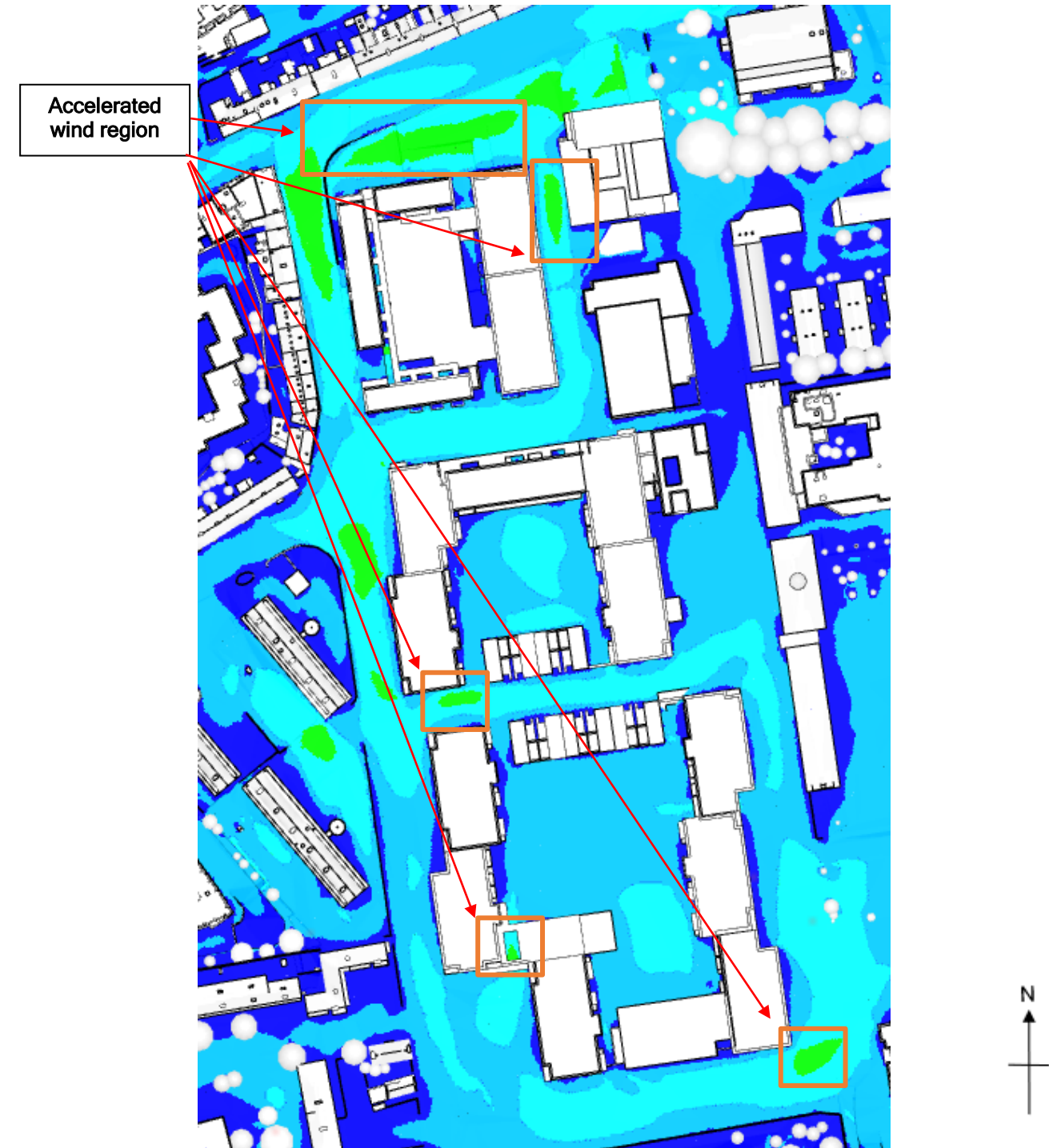
Fig. 4.1.2 – Lawson Criteria Results at 1.5m Above Ground Level Across Proposed Development
